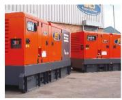
All generators are set to run at 50hz (1500rpm).
